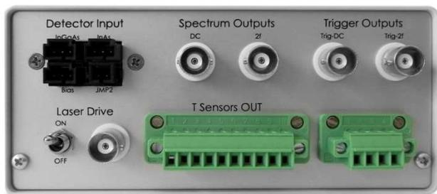
**Figure 1.** Front panel containing detector input connections, laser drive output, and outputs for spectra, triggers, temperature and pressure signals.
