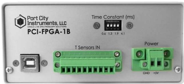
**Figure 2.** Back panel containing a DIP switch for time constant selection, USB type B port for flash programming, and screw terminals for power input and temperature sensor inputs.
